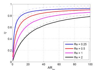
normalized charging power vs. PCM domain aspect ratio ( $AR_{xy}=L_x/L_y$ ) for different input powers ( $Q_{in} \sim Re$ ).
