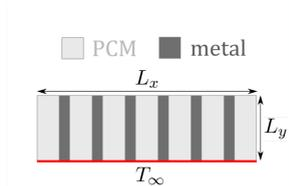
Highly conductive fins in a PCM domain heated by a constant wall temperature source
