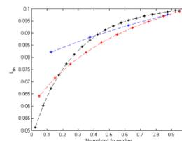
Optimised fin distribution for three cases (4, 10 and 20 fins) for the same input power, domain size and metal volume fraction: fin positions vs. normalised fin number
