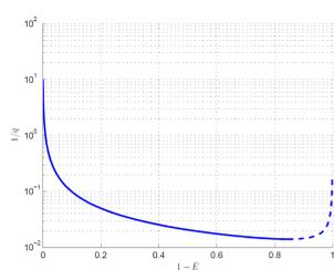
charging limits for infinitely thin fins showing the inverse power density vs. metal volume fraction.
