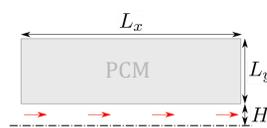
A PCM domain heated by a hot water flow with finite input power
